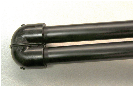
U-bend fabricated with butt-fused elbows
