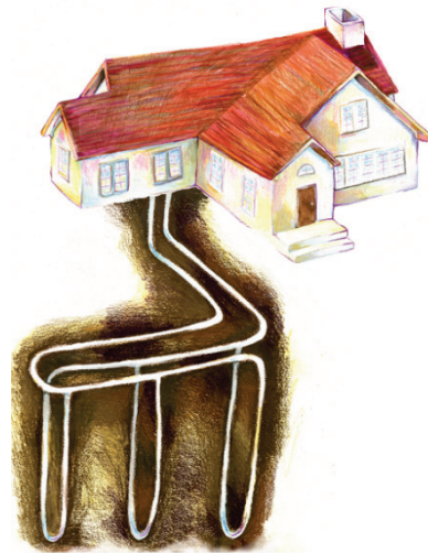
Vertical pipes in boreholes
