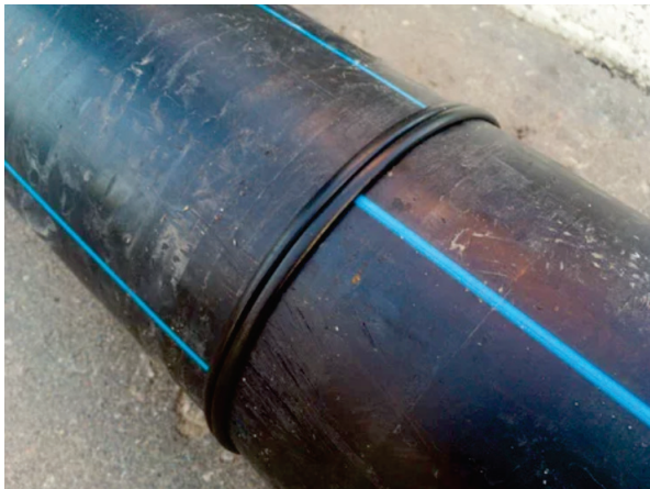
Butt fusion joint
